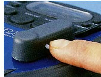
3. Activate the alert mode by pushing the anti-theft switch to alarm ON position
