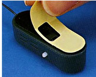
2. Peel the cover off the sticker on the sensor to expose adhesive and fix it to a flat surface on the product
