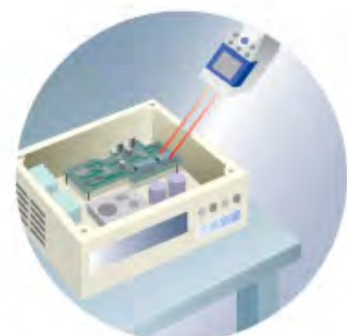
Surface temperature measurement of ICs and other minute surfaces
